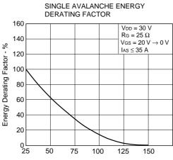
Starting  $T_{\text{ch}}$  - Starting Channel Temperature -  ${}^{\circ}\text{C}$
